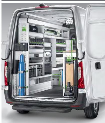
A unique feature of the systainer<sup>3</sup> storage case is that its integrated storage rails make it compatible with both cubio workshop and bott vario3 in-vehicle storage equipment. The most important tools and equipment are always to hand, neatly organised and easily accessible.
